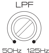
Fig.7 Low Pass Control (LPF)
