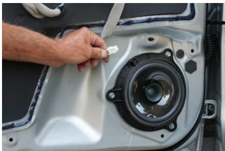
1. After removing the door panel, unplug speaker plug from factory speaker.
