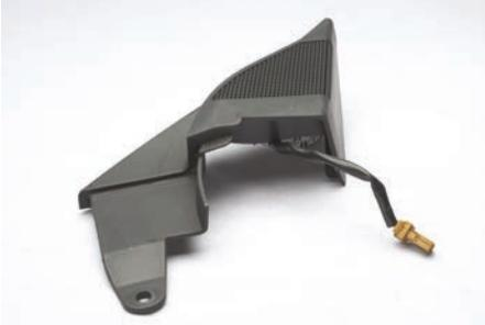
1. Remove door panel or unclip tweeter cover/housing to gain access to the factory tweeter.
