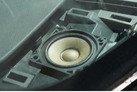
1. Remove factory grill from the vehicle to gain access to the factory tweeter.
