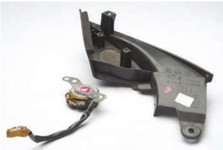
3. Remove factory bracket from tweeter and attach to new tweeter using the same hardware.
