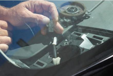
3. Locate both the tweeter adapter plate and the 2-pin tweeter plug adapter mount new tweeter in the adapter and connect the adapter plug (fig 2). Make sure the polarity is correct. Plug your new tweeter into the factory plug.
