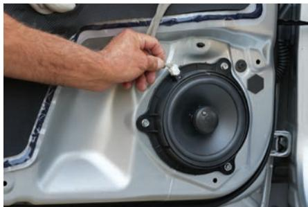
5. Now plug the factory speaker plug into the new speaker. If the factory plug is not long enough try to remove some of the tape on the wire to extend it or use the supplied extension cable (see Fig 4, pg 4). Reinstall door panel.
