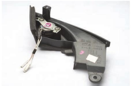
4. Locate the 2-pin tweeter adapter plug and connect it to your new tweeter (Fig 2), making sure the polarity is correct.
