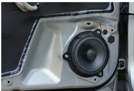
4. Fit new speaker in place and make sure all mounting holes line up. Install with the 3 x 10mm screws you removed from the factory speaker.
