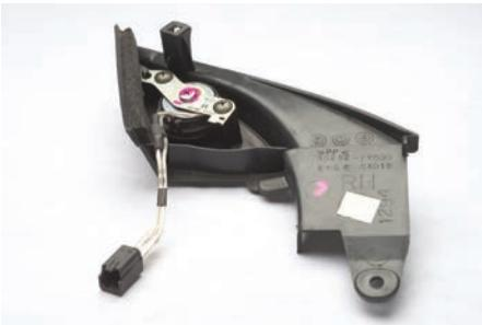
5. Plug your new tweeter into the factory plug and re-install door panel or tweeter cover/housing.
