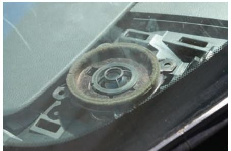
4. Install your new tweeter to the A pillar using the screws you removed from the factory tweeter. Reinstall factory grill.
