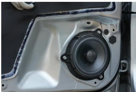
2. To remove the factory speaker, unscrew the 3 x 10mm bolts (do not discard these screws you will need them to install your new speaker)
