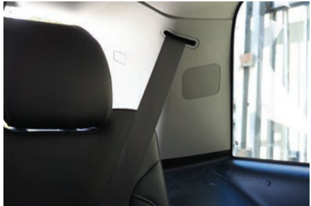
REAR 1. Remove panel to gain access to the factory speaker. Carefully unplug and remove panel and speaker.
