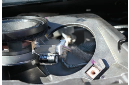
FRONT 2. Plug in and mount your new speaker with the screws you removed from the factory speaker.
