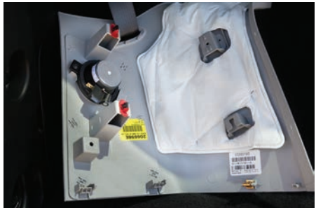
REAR 3. Mount your new speaker with the screws you removed from the factory speaker. Plug in and reinstall panel.
