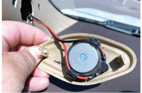
2. Unclip or remove factory tweeter from pillar or panel.
