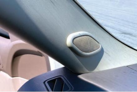
1. Remove pillar or panel to gain access to the factory tweeter, unplug and remove tweeter from the vehicle.
