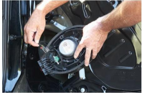
2. Remove the factory speaker by unclipping it at the top and pulling it forward. Then carefully unplug the speaker and remove from vehicle.
