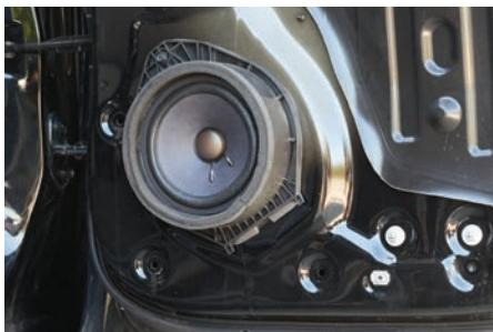
1. Remove door panel to gain access to the factory speaker. Remove the 7mm bolt at the top of the speaker (do not discard this bolt as you will need it to install your new speaker).
