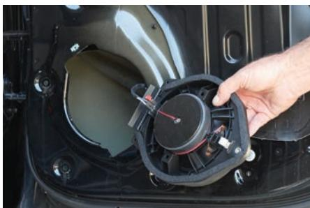
3. Plug in your new speaker and clip in starting from the bottom first. Securely mount the new speaker using the 7mm bolt. There are two extra mounting holes at the bottom of the speaker that will require drilling new holes to use. These are optional mounting holes
