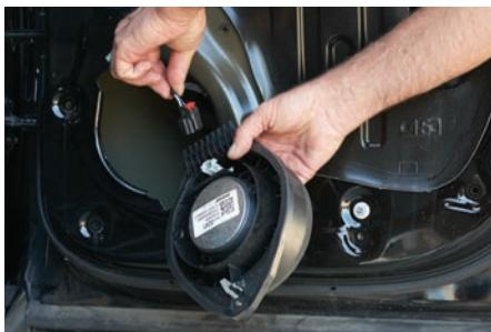
2. Remove the factory speaker by unclipping it at the top and pulling it forward. Then carefully unplug the speaker and remove the vehicle.
