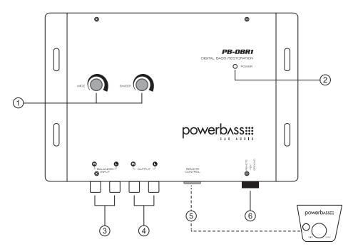
**1. WIDE** Adjusting this controls the width of the frequency range that will be restored. Minimum setting provides narrow width, Maximum provides a wide range.
