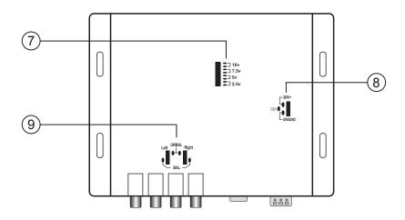
7. OUTPUT VOLTAGE CONTROL JUMPERS: The PB-DBR1 can either increase or decrease the output voltage of the Bass Restoration Circuit. Depending upon your system, you may change these jumpers to a higher or lower setting to maximize your output while protecting your speakers. In most systems the factory setting will be best all around.
