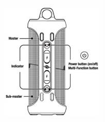
Long-press 'MASTER' and 'SUB-MASTER' (v) simultaneously for 2 seconds, you will hear prompt tone of power on. and they will begin to connect automatically. An audible beep will sound when connected successfully. The indicator light of SUB-MASTER will remain blue, and master indicator light flashes quickly.
