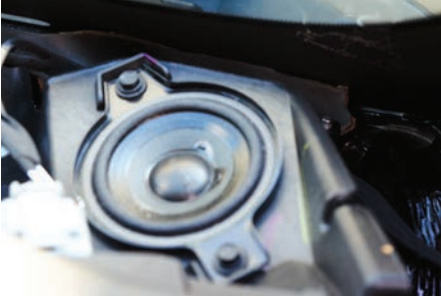
FRONT 1. Remove cover to gain access to the factory speaker. Remove the two 7mm screws securing the speaker. (Don't discard these screws as you will need them to install your new speaker) carefully unplug and remove speaker.
