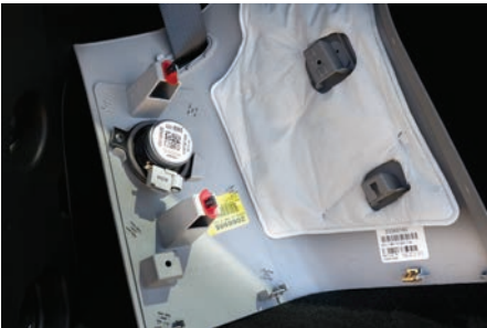
REAR 2. Remove one/two 7mm screws securing the speaker (Don't discard these screws as you will need them to install your new speaker) and remove speaker.
