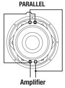
Parallel wiring a dual 4 ohm sub = 2 ohm
