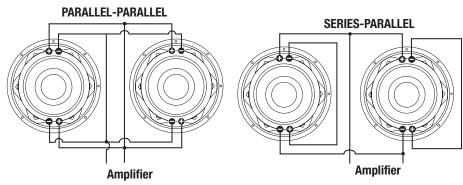
Parallel-Parallel wiring two dual 4 ohm subs = 1 ohm
