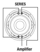
Series wiring a dual 4 ohm sub = 8 ohm
