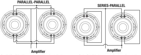
Parallel-Parallel wiring two dual 1 ohm subs = 1/4 ohm Parallel-Parallel wiring two dual 2 ohm subs = 1/2 ohm
