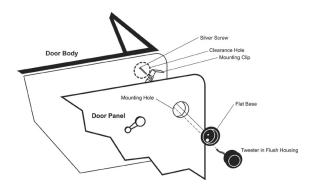
After checking for clearance, cut the mounting hole in the door panel (see Tweeter Specifications for hole size). Mount the Flat Base from the outside with the mounting clip on the inside of the door panel. Secure the mounting clip to the Flat Base with the long silver screw provided.
