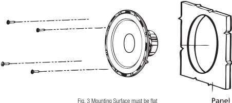
Fig. 3 Mounting Surface must be flat
