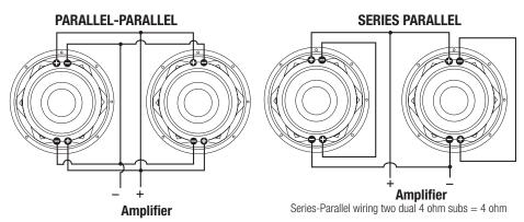
Parallel-Parallel wiring two dual 4 ohm subs = 1 ohm
