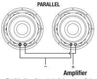
Parallel wiring of two single 4 ohm subs = 2 ohms
