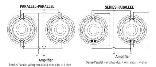
NOTE: Never connect only one coil of a Dual Voice Coil (DVC) speaker. BOTH voice coils must be connected to the amplifier
