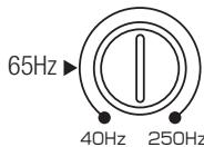
Fig.8 High Pass Control (HPF)
