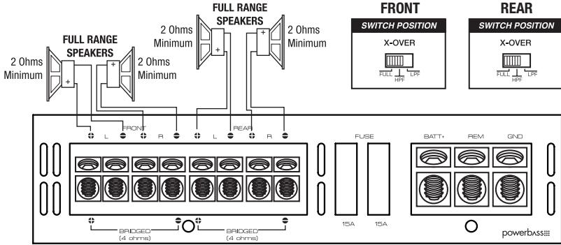
Fig.15 4-CH Speaker Connection / 2 ohms minimum
