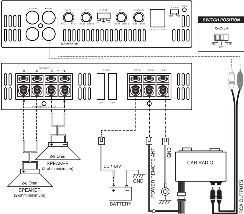
Fig.5 Low Level Input using RCA
