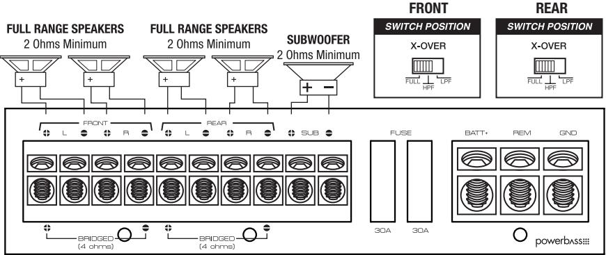
Fig.18 5-CH Speaker Connection / 2 ohms minimum
