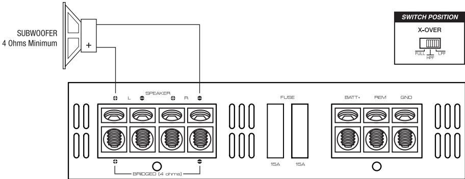
Fig.14 1-CH (Bridged Mode) Speaker Connection
