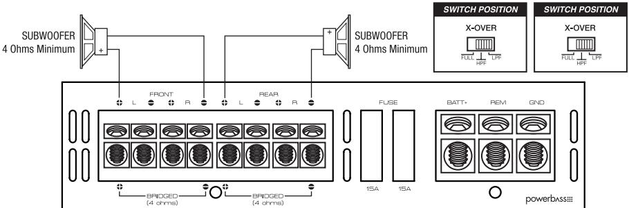
Fig.17 2-CH Speaker Connection / 4 ohms minimum
