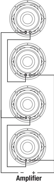
Series/ Parallel wiring of four single
