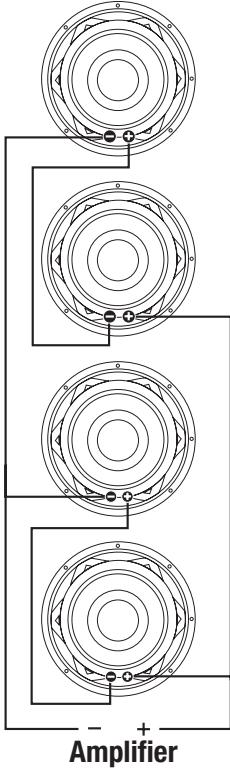
Series/ Parallel wiring of four single
