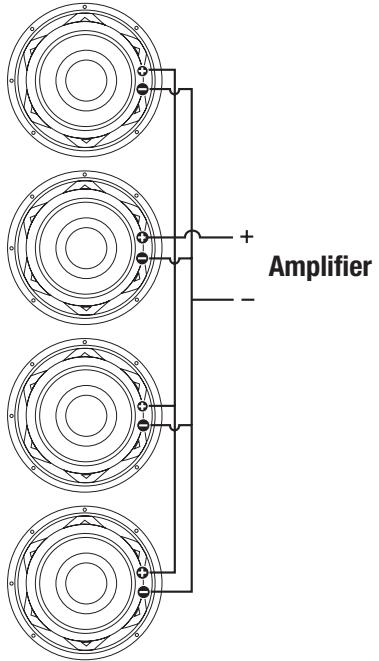
Parallel wiring of four single 4 ohm subs = 1 ohms
